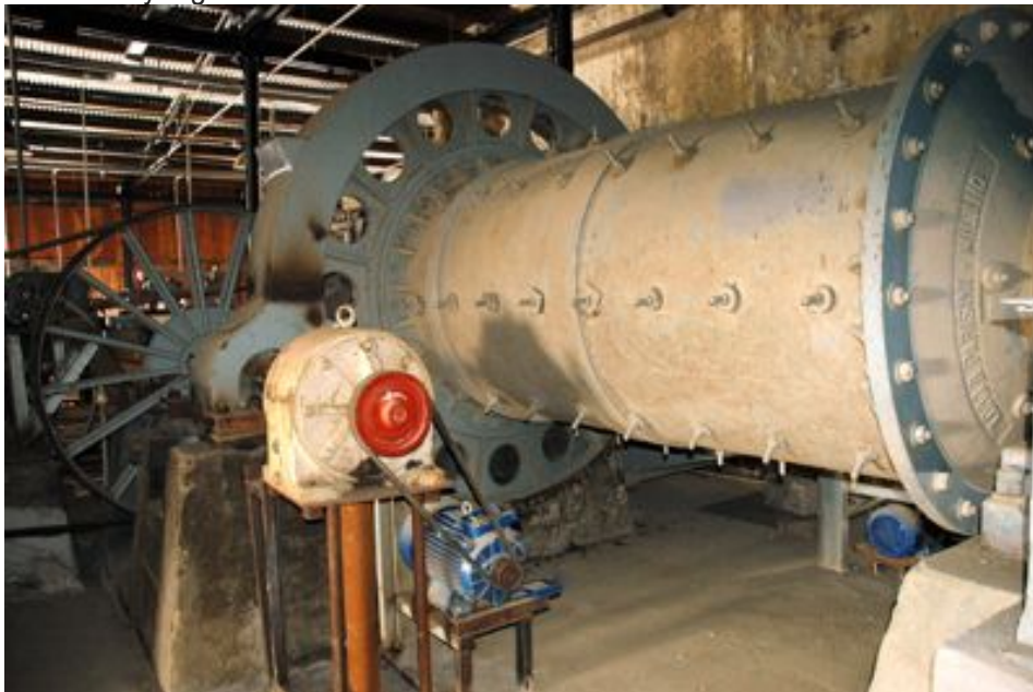
foto 5: Rosas washing plant: the ball mill
